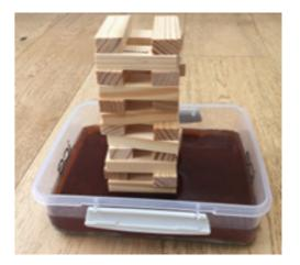
The above tub was approx. 230mm by 170mm (2litre capacity) and required 5½ packs of plasticine for a 10mm deep layer. Two packets of jelly making approx. 1 litre, gives a sufficient depth of "unstable ground".
